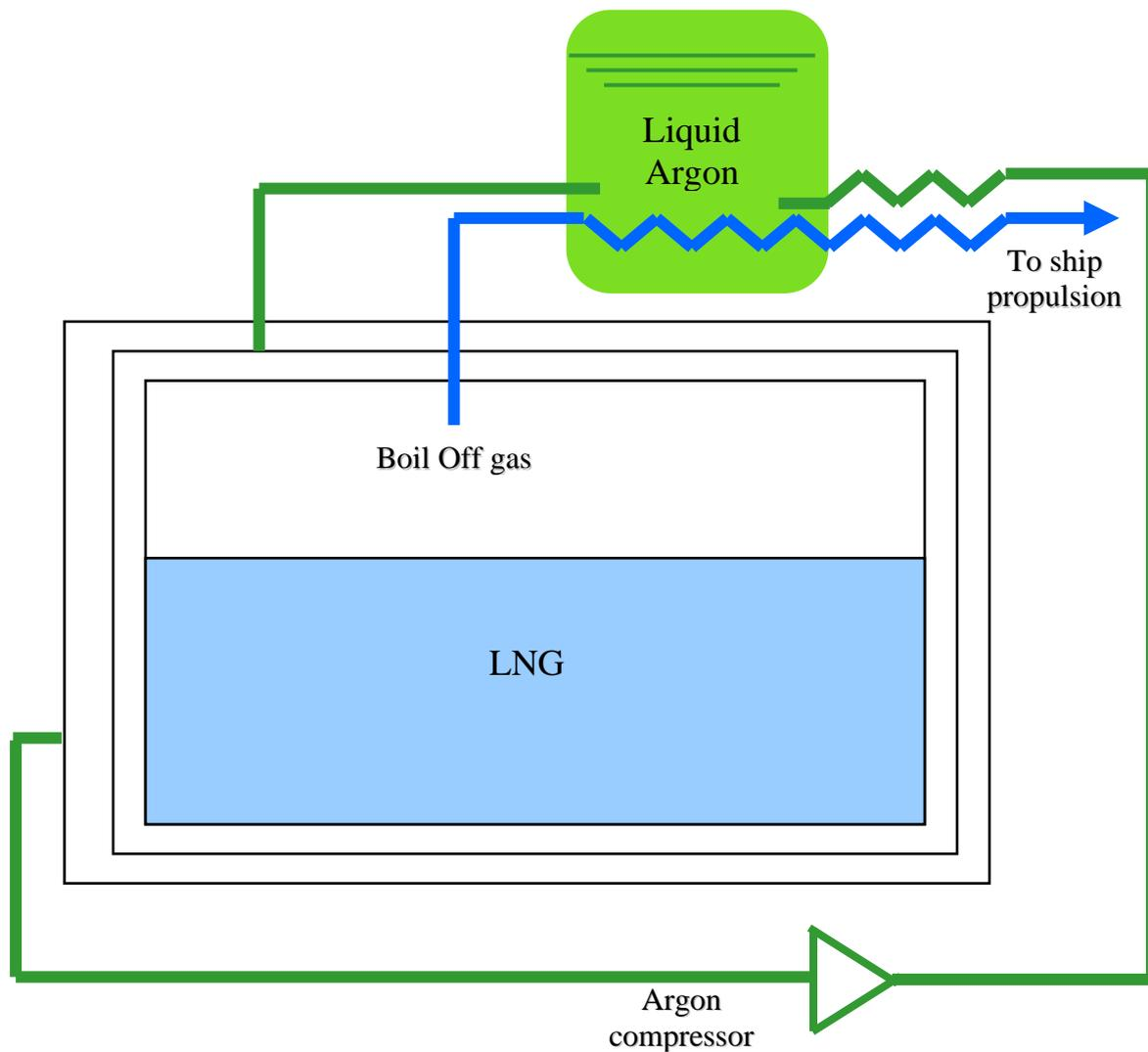
**Figure 8: Closed loop argon supply configuration**
