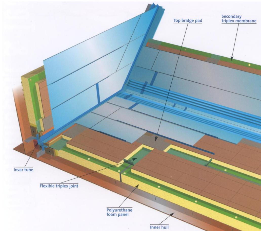
**Figure 3 : CSI foam insulation by Gaz Transport and Technigaz**
