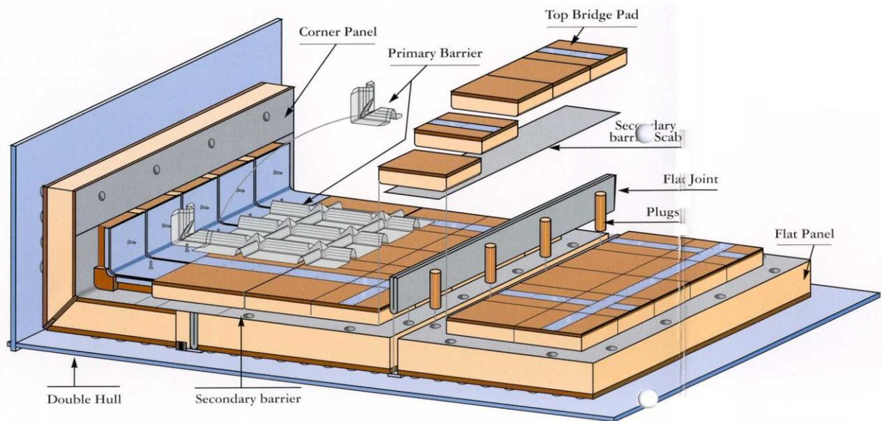
***Figure 1 : Mark 3 type foam insulation proposed by Gaz Transport and Technigaz***
