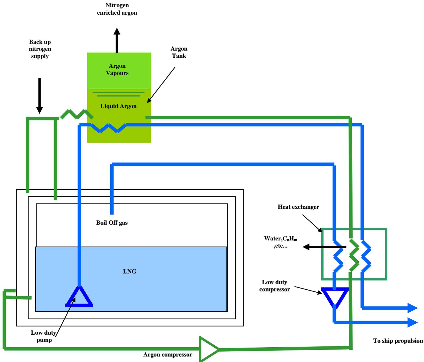
***Figure 9 : Argon purification system***
