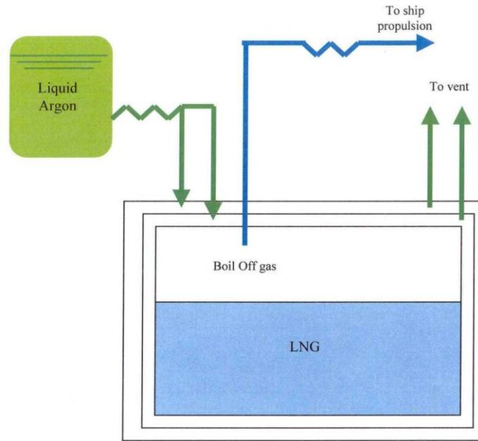
**Figure 5 : Open loop argon supply configuration**
