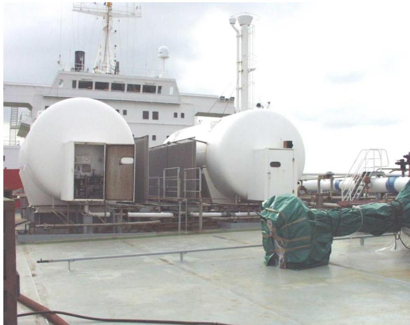
**Figure 6 :Example of on board liquefied nitrogen storage tanks and vaporisers which could be directly used to store liquefied argon.**
