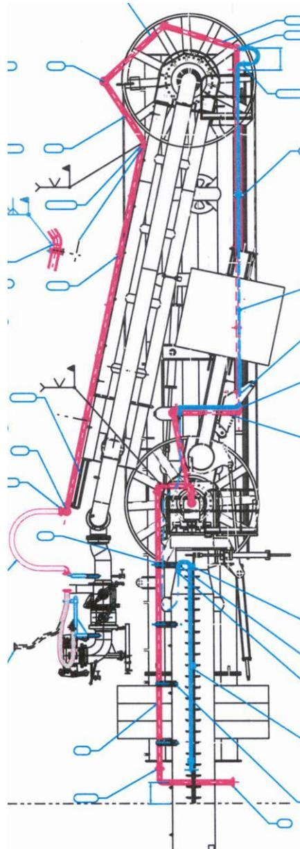
**Figure 7 : Example of Liquefied nitrogen loading lines (in red) attached to an LNG loading arm, proposed by FMC loading systems, which could be directly used to supply liquefied argon**
