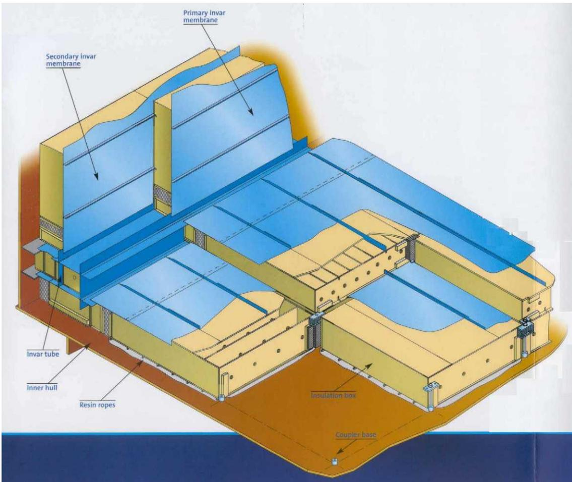
**Figure 2: NO 96 perlite insulation by Gaz Transport and Technigaz**
