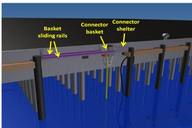
**Fig. 6** PLUG typical quay side implementation
