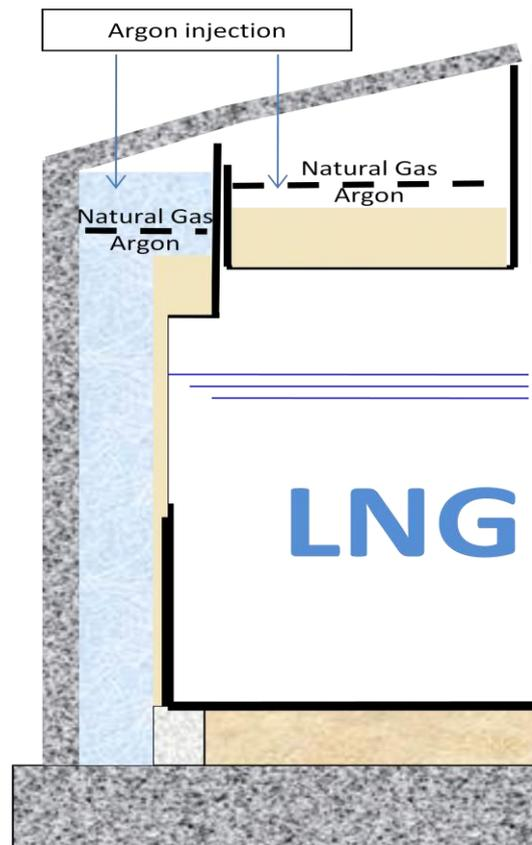
**Figure 3 : Typical LNG storage tank argon insulation implementation**
