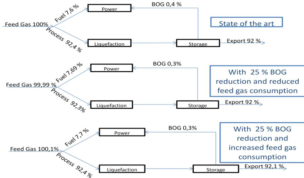
**Figure 4 : Benefit for liquefaction plant process flow**
