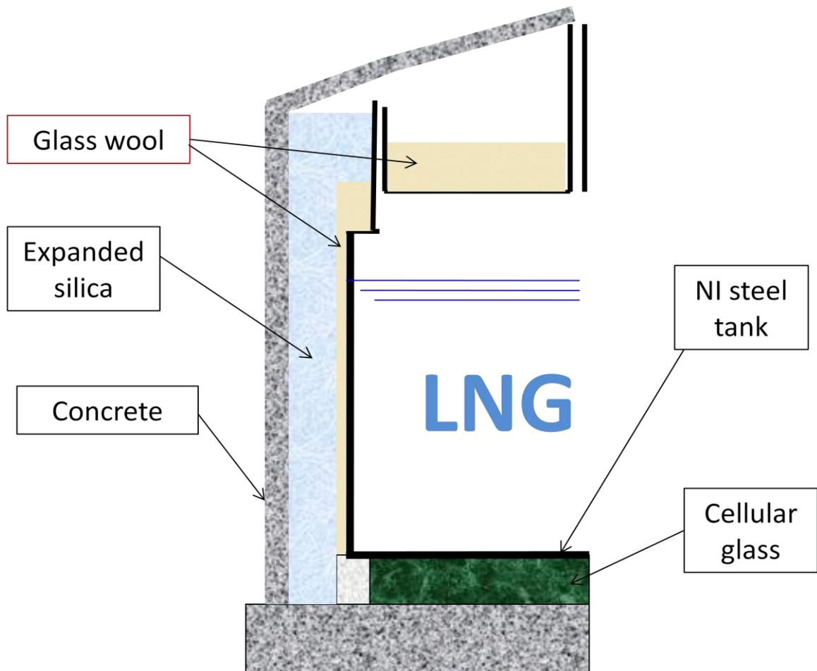
**Figure 1: Typical LNG storage tank configuration**
