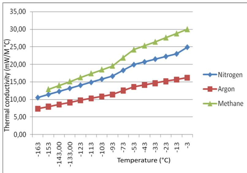
**Figure 2 : Nitrogen, Methane and nitrogen thermal conductivity**
